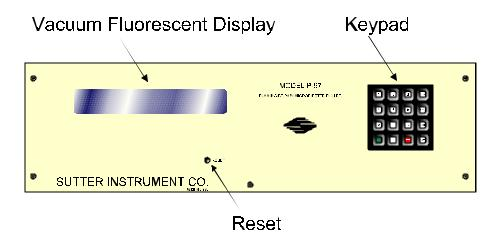
Figure 5. P-97 Front Panel
