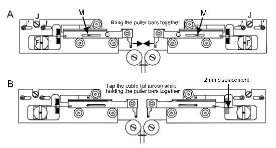
Figure 26. Pulley Adjustment
