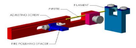
Figure 20: Fire Polish Spacer in Puller Bar
