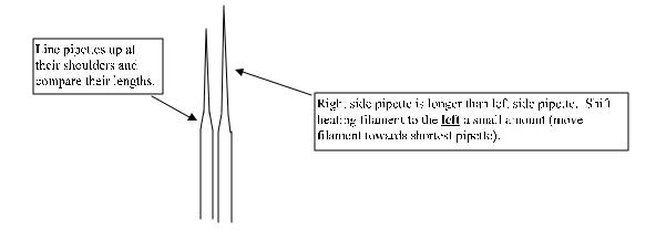
Figure 25. Micropipette Shapes
