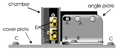
Figure 8. Filament Block Assembly
