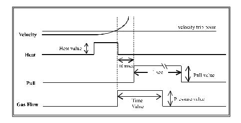
Figure 10. Pull Cycle when TIME > 0
