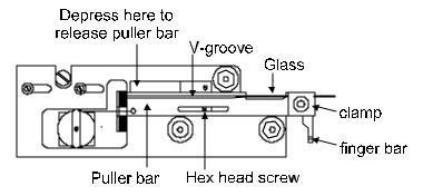
Figure 4. Left Puller Bar
