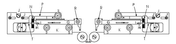
Figure 9. Upper Cable Pulley Assembly
