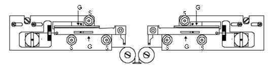
Figure 23. V-groove Bearings and Puller Bars
