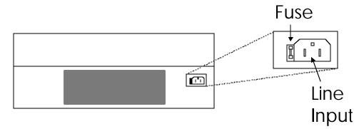
Figure 1. P-97 Cabinet (rear view)
